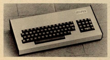
This new MKB-2 keyboard is designed for use with the 64 and 80 character display video boards. Standard features on the MKB-2 include: a numeric key pad, upper and lower case, cursor control keys, 2 key rollover, and automatic repeat on all keys. The MKB-2 is assembled in a heavy duty steel case with parallel interface, strobe or pulse and on board regulation (5 V, 12 V), and comes complete with standard DB25S connector and black double injection molded keys.
