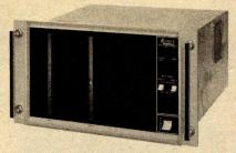
The new Remex-11 floppy disk systems are integrated hardware and software units that connect directly to the PDP-11 Unibus or LSI-11 Q bus. The systems are available with a utility function that permits data interchange between IBM 3740 diskettes and any RT-11 supported device.
