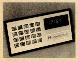
Compucruise is an automotive microcomputer combining a 20 button backlighted keyboard, 5 digit blue fluorescent display, and appropriate sensors to provide a fuel management system, trip computer, clock and digitally displayed cruise control. Compucruise monitors speed, distance, fuel flow, time, battery voltage and choice of three tempera-
