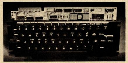
This new solid state keyboard uses a second generation microprocessor and low profile capacitive keyswitches. The keyboard uses an 8 bit single integrated circuit processor with on chip read only memory, programmable memory and erasable read only memory. All key functions are software controllable. The microprocessor permits automatic repeats, multiple application programs in a single intelligent encoder, field program changes using new firmware,
