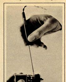
The Soldercraft Model 6A is a miniature low voltage production soldering iron designed for versatile microcircuit and fine instrument work. This soldering iron, when powered by a multitap 18 W low voltage transformer, will provide controlled temperatures of 700° F at 6 V, 625° F at 5.5 V, 555° F at 5 V and 480° F at 4.5 V from its 3/32 inch (0.25 cm) tip. The heat is generated entirely within the tip, which provides maximum efficiency and faster heat recovery.
