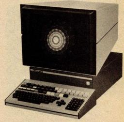
Chromatics Inc has introduced the CG series line of full 8 color graphic and alphanumeric readout computers. The line consists of 13, 15 and 19 inch models featuring noninterlaced screen refresh, high resolution shadow tubes, and 512 by 512 or 512 by 256 individually addressable and color selective dots. Each model employs a Z-80 processor with full memory and input and output (IO) structure. The 13 inch model starts at \$8995.
